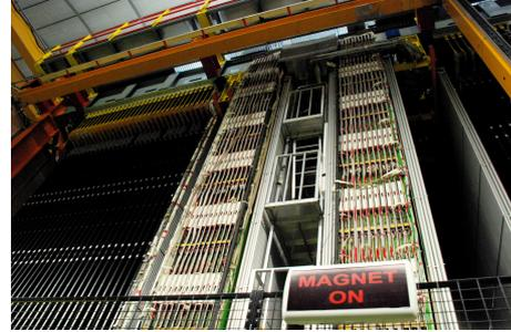
**Figure 3.19:** Photograph of the OPERA spectrometer of SM 1. The first target section is visible on the left.
