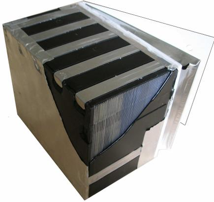
**Figure 3.14:** Photograph of a partially opened OPERA ECC brick. The detached CSD, separately packed in aluminum, is visible on the right side in the opened white plastic box.
